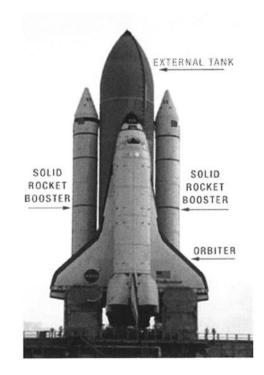
Figure 4.1.1-1. The principal components of the Space Shuttle. Source: NASA
